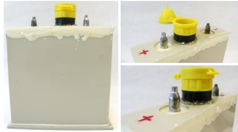
Fig. 5. Example of a flooded 2 V/ 22 Ah cell.
